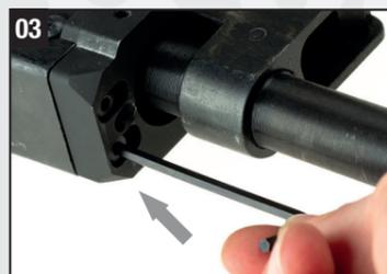
**03** Tighten both locking screws with suitable tool.
