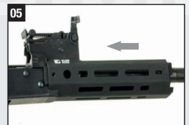
**05** Push the front assembly block forward until the threaded hole is visible.
