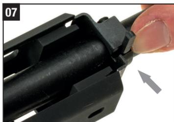
**07** Move the fore-end cap until the locking lever can be folded down.
