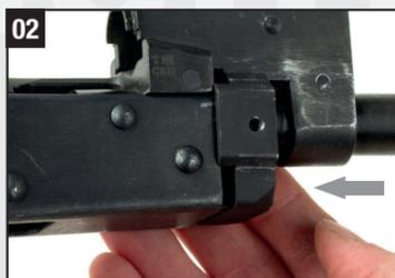
**02** Place the retainer onto the housing.
