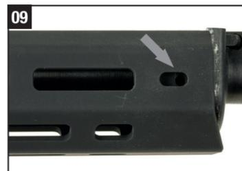
**09** Move the front assembly block until the threaded hole is visible.
