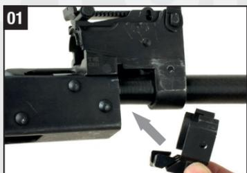
**01** Dismantle AK original parts and prepare for mounting the rear holding block.
